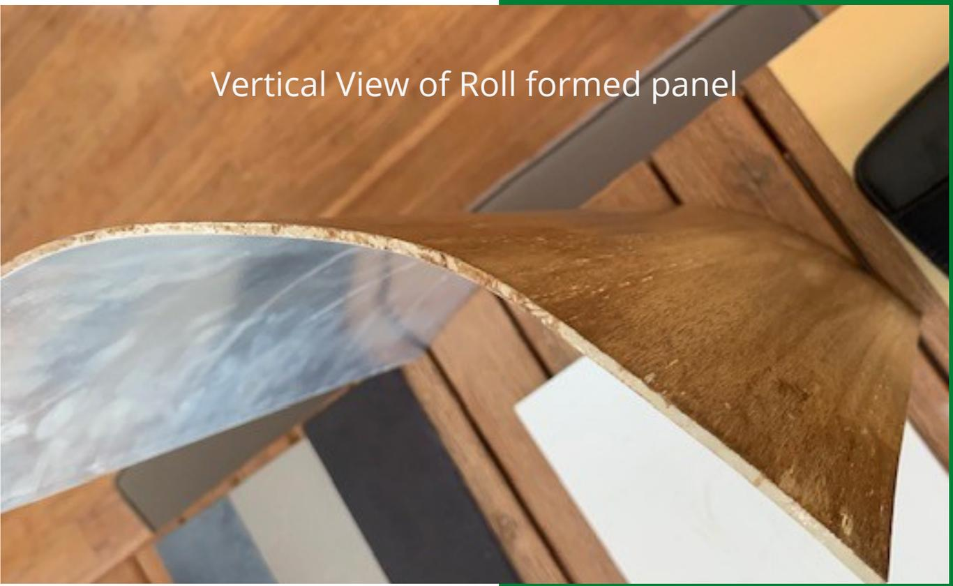
Maximum sheet size is 3000mm x 1500mm and can be factory cut to suit site panel sizes.
